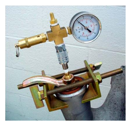
Use a gage and wristwatch to measure pressure loss over time.
