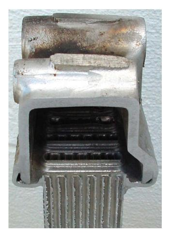
Stress cracking tends to occur in the lighter gage components. Here's an actual crack in the tube-to-header joint. Hint: look on the right side.
