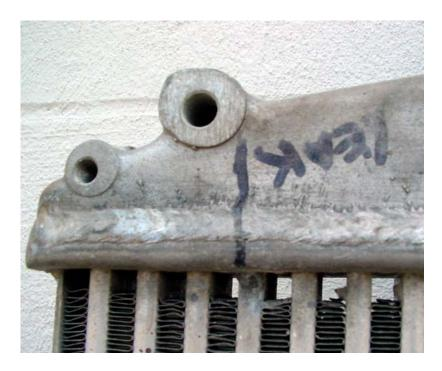
Pressure loss will occur through almost invisible cracks.
